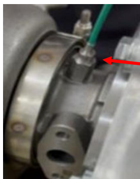
Tighten speed sensor to 15.0 – 17.0 Nm
