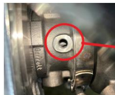
Above pictures show bearing spacer hole not aligned with center housing hole.
