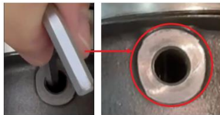
Above pictures show bearing spacer hole aligned with center housing hole.
