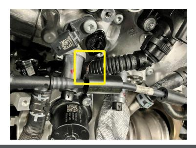
3. Tape should be used in the area where the wire shroud is close to the engine block for wear protection.
