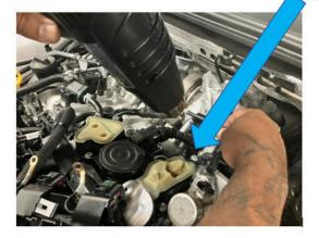
2. To elongate the venturi injector wire heat shroud, apply gentle heat approx 2-3 inches (5-15cm) away from the wire heat shroud until shroud can be elongated to desired length.
