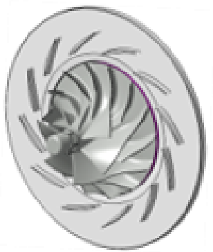
Compressor wheel w/ vane diffuser
