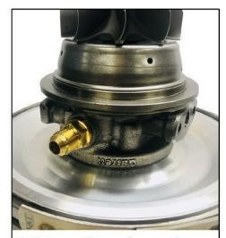
Fig B: New turbine aero has a peak efficiency of 77% and flows 10% more than GTX42. Aluminum backplate helps reduce weight. -6an water fittings come installed.
