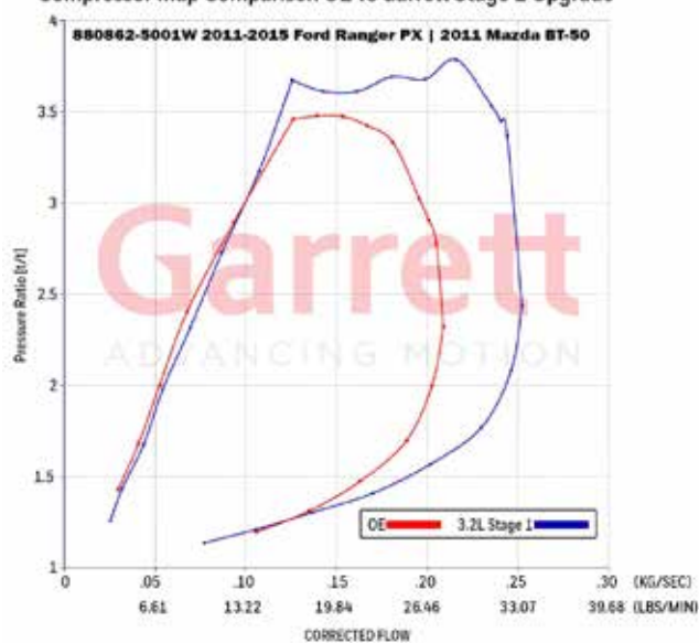
Compressor Map Comparison OE vs Garrett Stage 1 Upgrade
