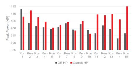
Vehicle dyno test data comparing OE to Garrett. Multiple back to back dyno pulls measure intercooler effectiveness by comparing horsepower output...
