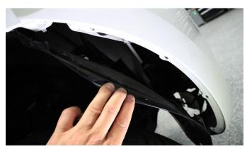
8. Separate the lower air dam from the bumper by removing the (4) 10mm bolts along the bottom of the bumper.
