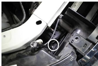
5. With a T-25 torx bit, remove the (2) screws attaching the grill to the bumper. These can be reached from the lower grill opening.
