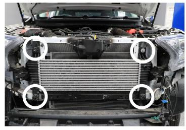
16. Remove rubber bushings from the OEM intercooler. Use caution not to tear the rubber. First push out the metal sleeve from all (4) bushings. Next gently roll the bushing out of the tab. Once all (4) bushings are out, put the bushings and sleeves into the Garrett Intercooler Core. Your Garrett cores is ready to be installed.
