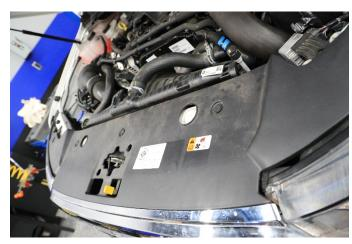
2. Once the pop clips are removed, tilt the rear of the air dam up. Reach an arm under the air dam towards the grill and locate the (4) tabs that attach the air dam to the grill. Unlock the tabs and remove the air dam. Use extra caution not to break off the tabs.
