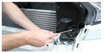
11. Starting with the wheel well sides of the bumper, gently unclip the bumper from the fender. Follow the process and work your way towards middle of the grill to detach all points. You are now ready to remove the bumper. Using a helper, support the bumper at each corner and simultaneously separate the bumper from the truck. Ensure no wires are connected as the bumper is separated. Set in a place where the bumper will not get scratched.
