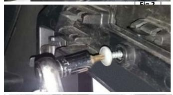
6. There are (4) plastic locking tabs holding the lower grill to the bumper. From the lower bumper opening, locate these tabs and carefully release them. There are (2) additional tabs per side that will need to be released as the grill is removed. Remove grill and detach all locking tabs.
