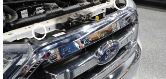
4. Using a ratchet with a long extension and 10mm socket, remove the (2) lower bolts behind the headlights.
