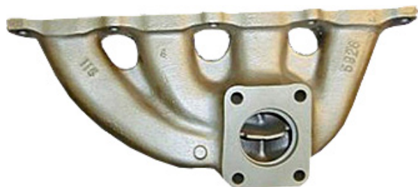
Figure 5. Cast manifold with a divided turbine inlet design feature
