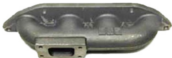
Figure 3. Cast log style turbocharger manifold
