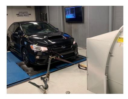
Multiple back-to-back dyno pulls in a wind tunnel to simulate real world driving conditions.
