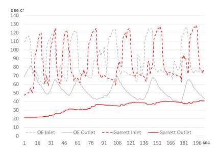
Vehicle dyno test data comparing OE to Garrett. Multiple back to back dyno pulls measuring inlet and outlet temps to compare intercooler effectiveness and heat saturation point.
