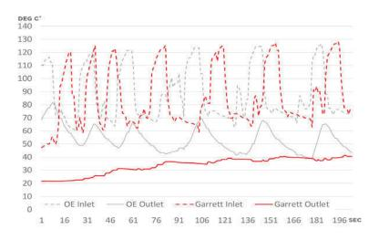
Veicle dyno test data comparing OE to Garrett. Multiple back to back dyno pulls measure inlet and outlet temps to gauge intercooler effectiveness and heat saturation point.
