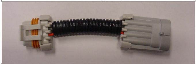
Use This Adapter on Model Year 2004 and 2005 vehicles to convert the vehicle wiring harness to the updated Vane Position Sensor included on the Upgrade Turbocharger. For the Model Year 2006 and newer, this adapter is not needed and may be discarded.
