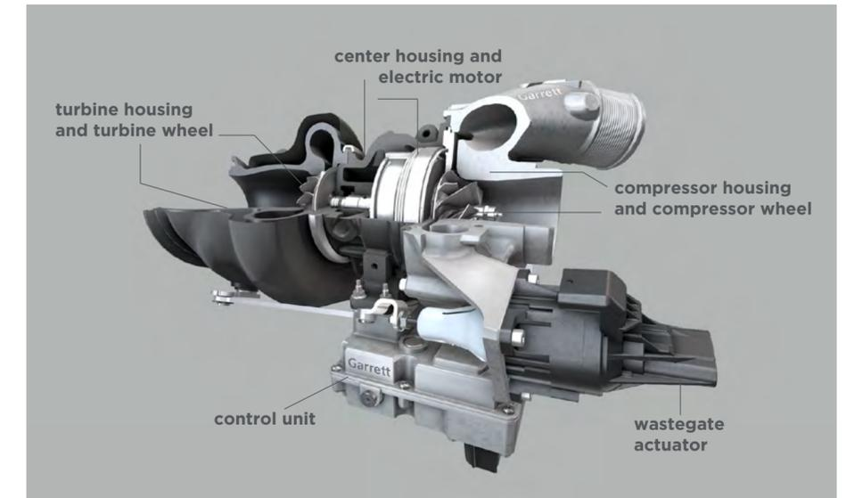
Turbochargers use otherwise wasted exhaust energy that would exit the tailpipe to drive a turbine wheel connected via a shaft to a compressor wheel. The compressor wheel packs more air into the engine yielding the "turbo boost" to vehicle acceleration. This has allowed automakers to use smaller, more efficient engines helping to improve fuel efficiency and reduce carbon dioxide emissions without compromising performance.
